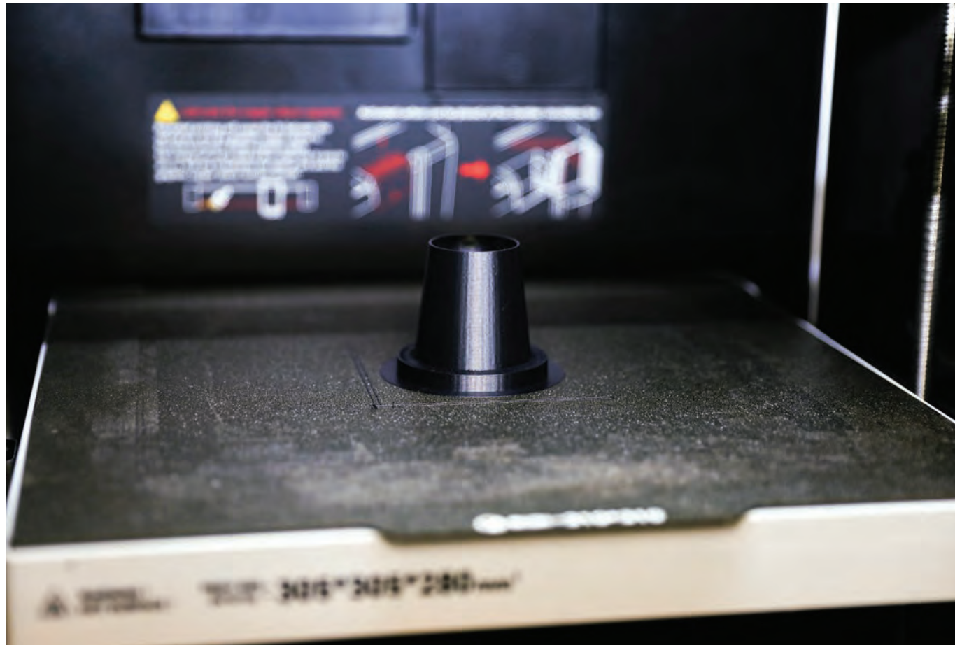
A 3D-printed protective sleeve rests on the print bed after fabrication by Allied Trades Soldiers assigned to the 325th Light Support Battalion, 3rd Mobile Brigade, 25th Infantry Division, during Joint Pacific Multinational Readiness Center 26-01, Nov. 4 2025, Schofield Barracks, Hawaii. (Photo by SSG Andre Taylor)
